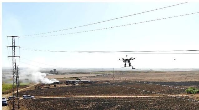
FIGURE 2. Aerial manipulation robot approaching to a 15 kV power line.
