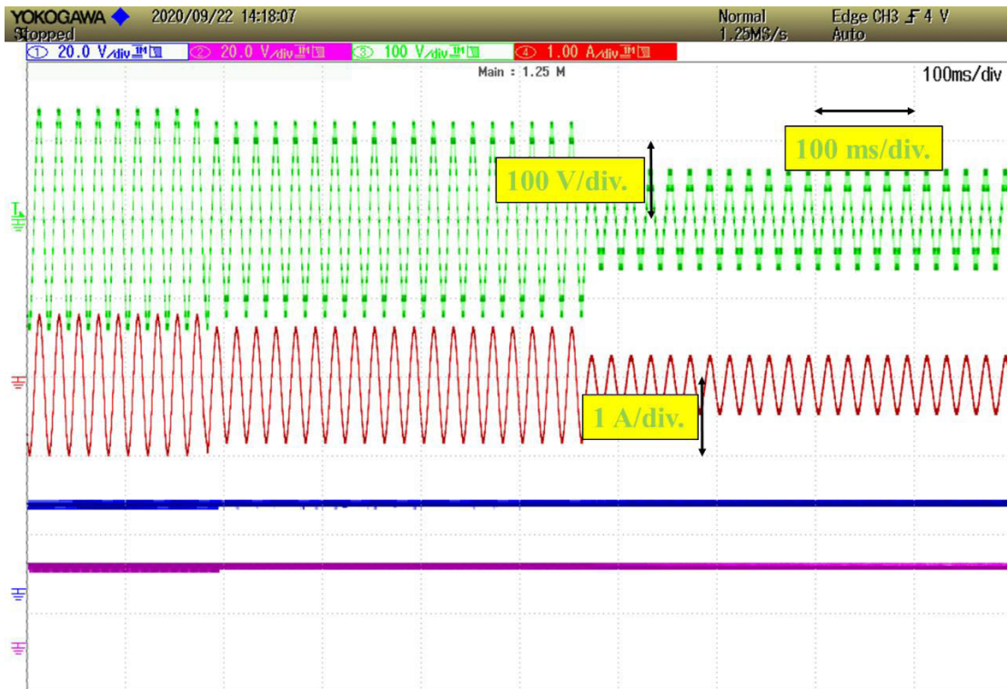
FIGURE 13. Output waveform for dynamic alteration of modulation index.
