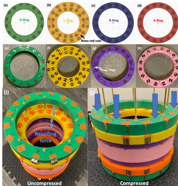
FIGURE 4. Construction and assembly of the Halbach magnet. Photos of the four (out of 8 total) designed (a-d) and manufactured (e-h) formers. The other four rings (not shown) are identical. The 3D printed formers with N40UH blocks fitted into former pockets are shown. Eight cylindrical (6.35 mm diameter) cuts in the CAD models allow throughput for brass rods, and the pegs/holes in formers minimize ring shifting when compressed. (i-j) Flange brass nuts are tightened, compressing the rings (blue arrows) into their optimized geometry.
