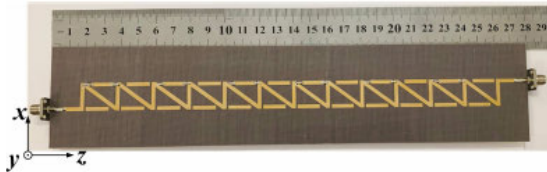
FIGURE 34. Reconfigurable microstrip LWA with a staggered strip line [109].
