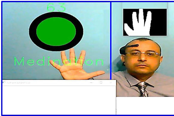
FIGURE 13. Entering one bit with "0" value by opening hand and relax.
