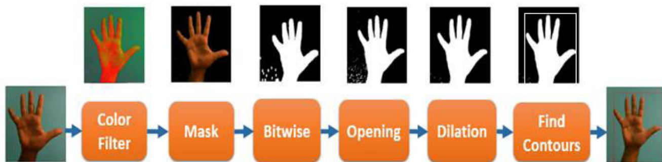
FIGURE 8. Steps for hand detection.
