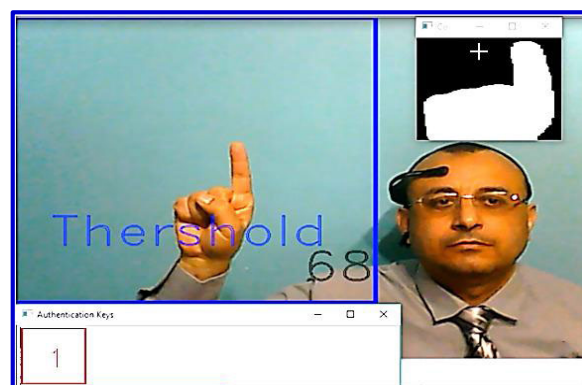
FIGURE 12. Selecting the attention threshold value by raising the index finger.
