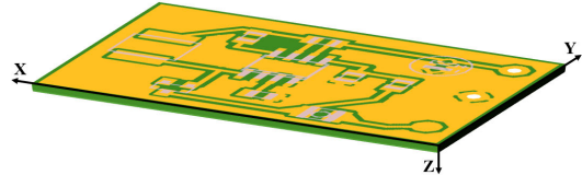
FIGURE 1. Structure schematic of a rectangular PCB with one core.
