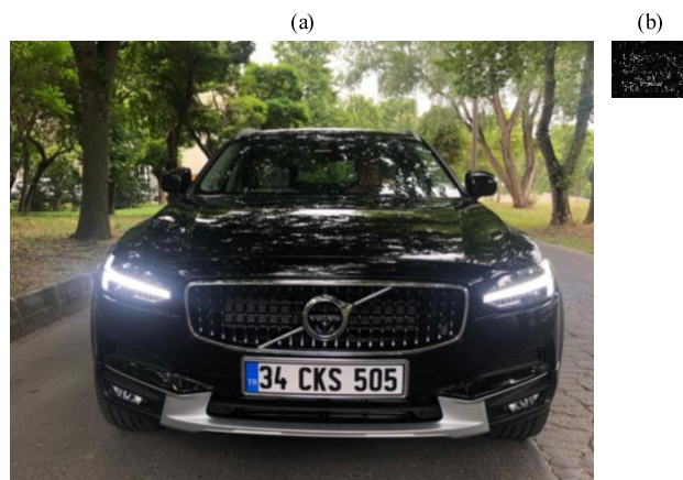
FIGURE 7. The size of the compressed domain image in comparison to the size of the pixel domain image. a) A 1024 \times 768 pixel domain image. b) A compressed domain image corresponding to the pixel domain image with a resolution of 128 \times 96 pixels, where each CU is represented by a single pixel.
