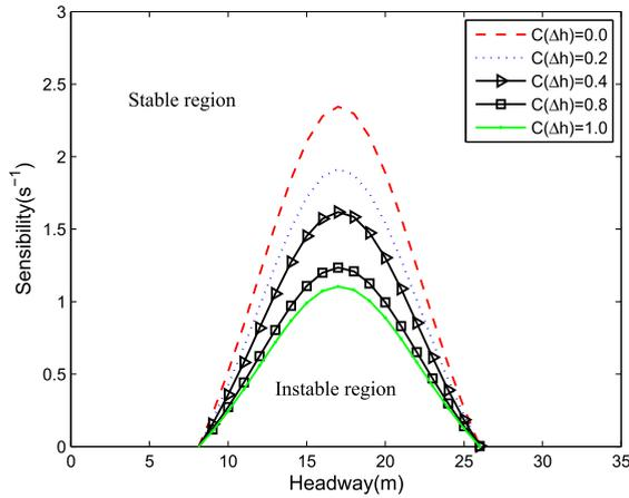
FIGURE 4. Neutral stability curves with different cooperative level  $C(\Delta h)$  for lane-changing mode.
