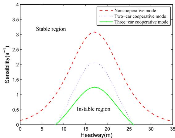
**FIGURE 3.** Neutral stability curves with different cooperative vehicles  $n$  for non-lane mode.
