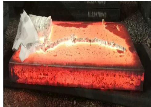
FIGURE 4. The state of the test slab after discharging out from the furnace.
