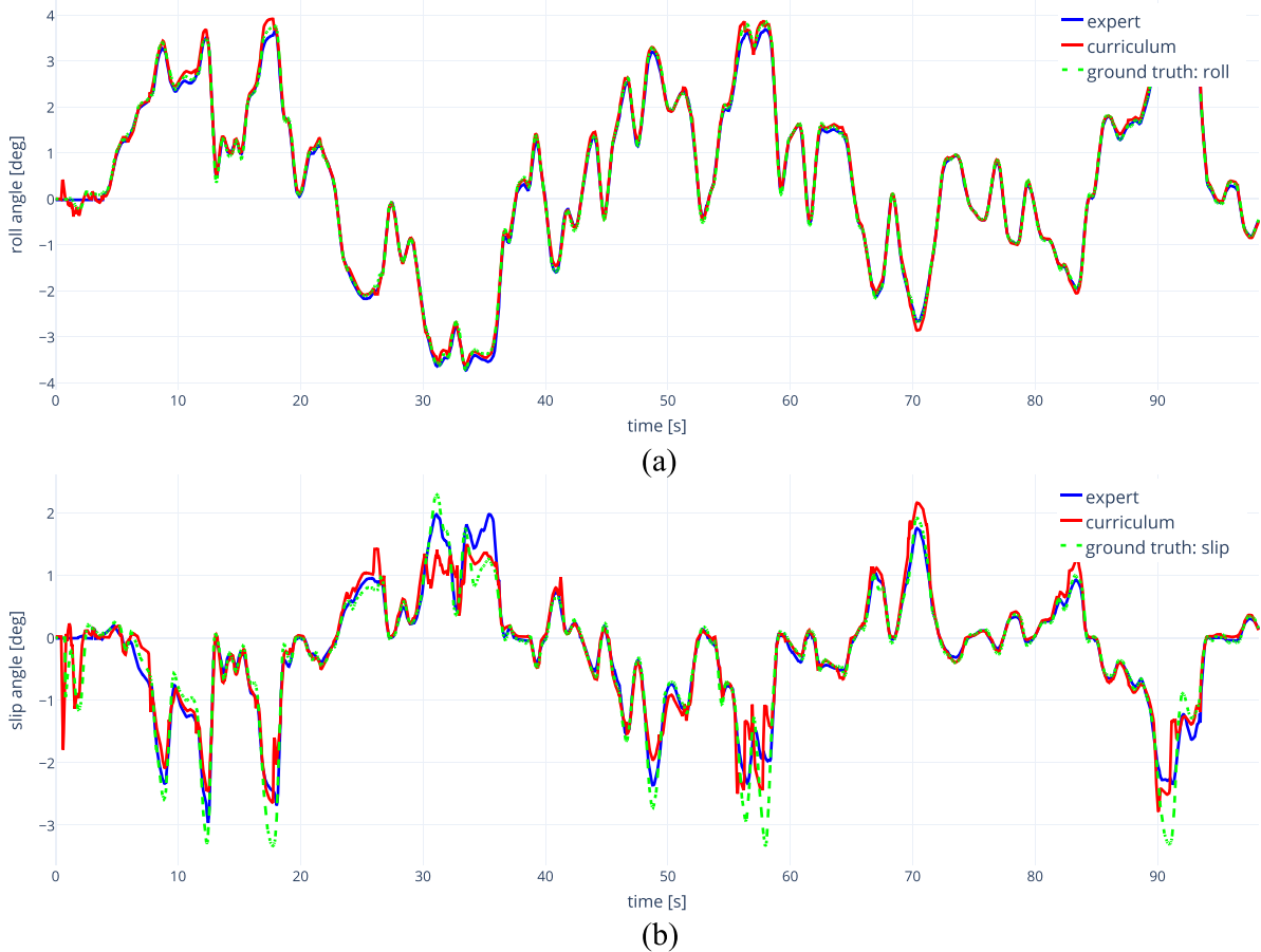
FIGURE 11. Inference results of our model and the expert model. This validation data were acquired from a human driver on a road with a friction coefficient of 0.85 and a desired vehicle speed of 80 km/h. (a) Roll angle predictions graph, and (b) sideslip angle predictions graph.
