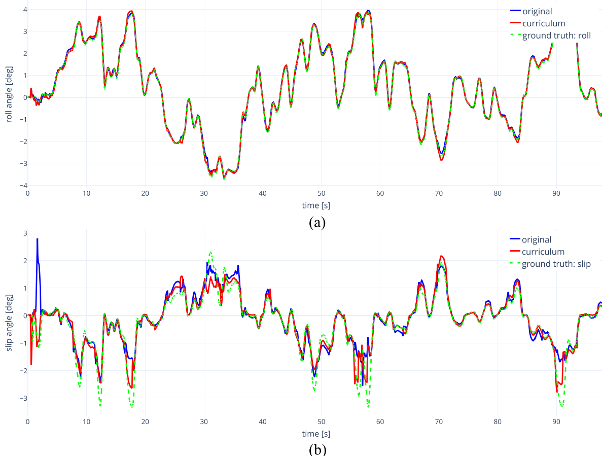
FIGURE 6. Inference results of non-curriculum and curriculum methods on a maneuver at a race track by the skilled human driver. The validation data were acquired on a road with a friction coefficient of 0.85 and a desired vehicle speed of 80 km/h. (a) Roll angle predictions graph, and (b) sideslip angle predictions graph.
