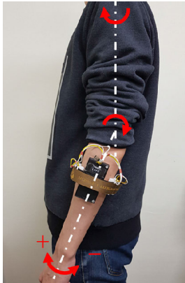
(b) The arm swing configuration while wearing the haptic bracelet
