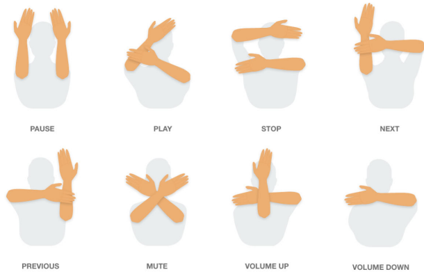
FIGURE 10. Gesture protocol related with Pause, Play, Stop, Next, Previous, Mute, Volume Up, and Volume Down.
