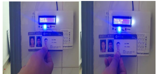
(c) LCD displays name and student’s number of first card (d) LCD displays name and student’s number of second card
