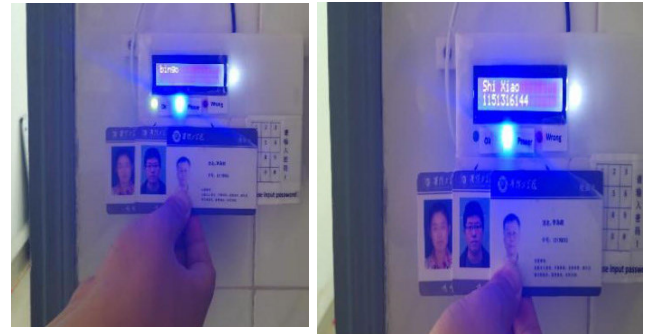
(a) LCD displays “bingo” (b) LCD displays name and student’s number of first card
