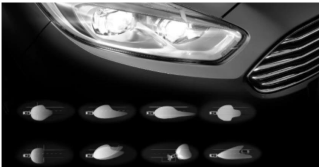
FIGURE 13. Beam patterns for projections in the ford AFS [14].
