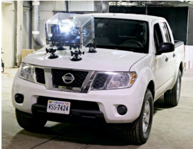
FIGURE 12. The headlamp experimental setup on a vehicle [11].
