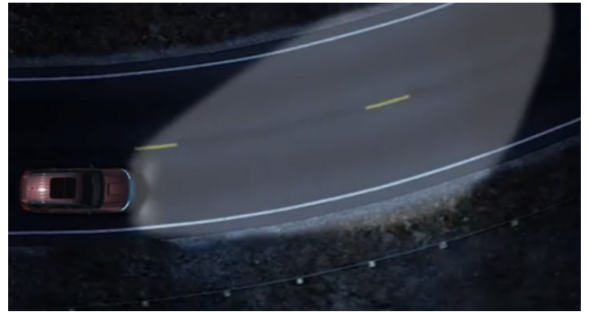
FIGURE 14. The beam projections across a curve in the ford AFS [14].
