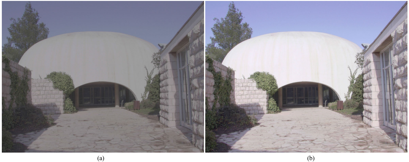
FIGURE 2. Tone-mapped LDR versions of the HDR image “dani_synagogue”: (a) the LDR image from the default TMO of JPEGXT profiles A and C; (b) the dynamic range of the image in (a) is linearly stretched to the full 0 – 255 range.
