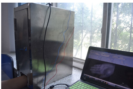
FIGURE 10. Inside box palm vein image capture device.
