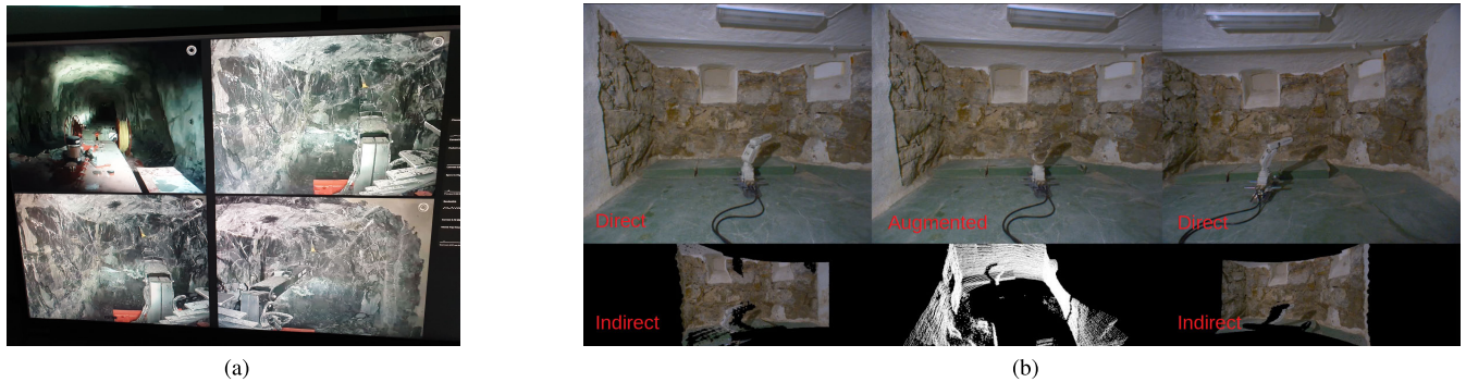
FIGURE 1. (a) Remote operation interface for a scaling machine in a Swedish mine, showing direct rendering of on-vehicle camera views. Photo provided by Boliden AB. (b) Remote operation interface of the proposed system, showing rendering of direct, indirect, augmented and lidar views.
