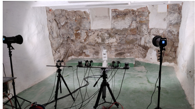
FIGURE 3. Test scene setup with cameras and lighting, with remotely actuated robotic arm as in-scene occluder.
