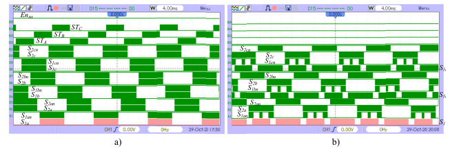
FIGURE 18. Switching and control signal generation a). Digital outputs from RT box 1. b) Control signals from PCB.
