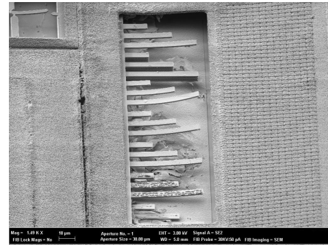
(a) Damage to the standard passivation
