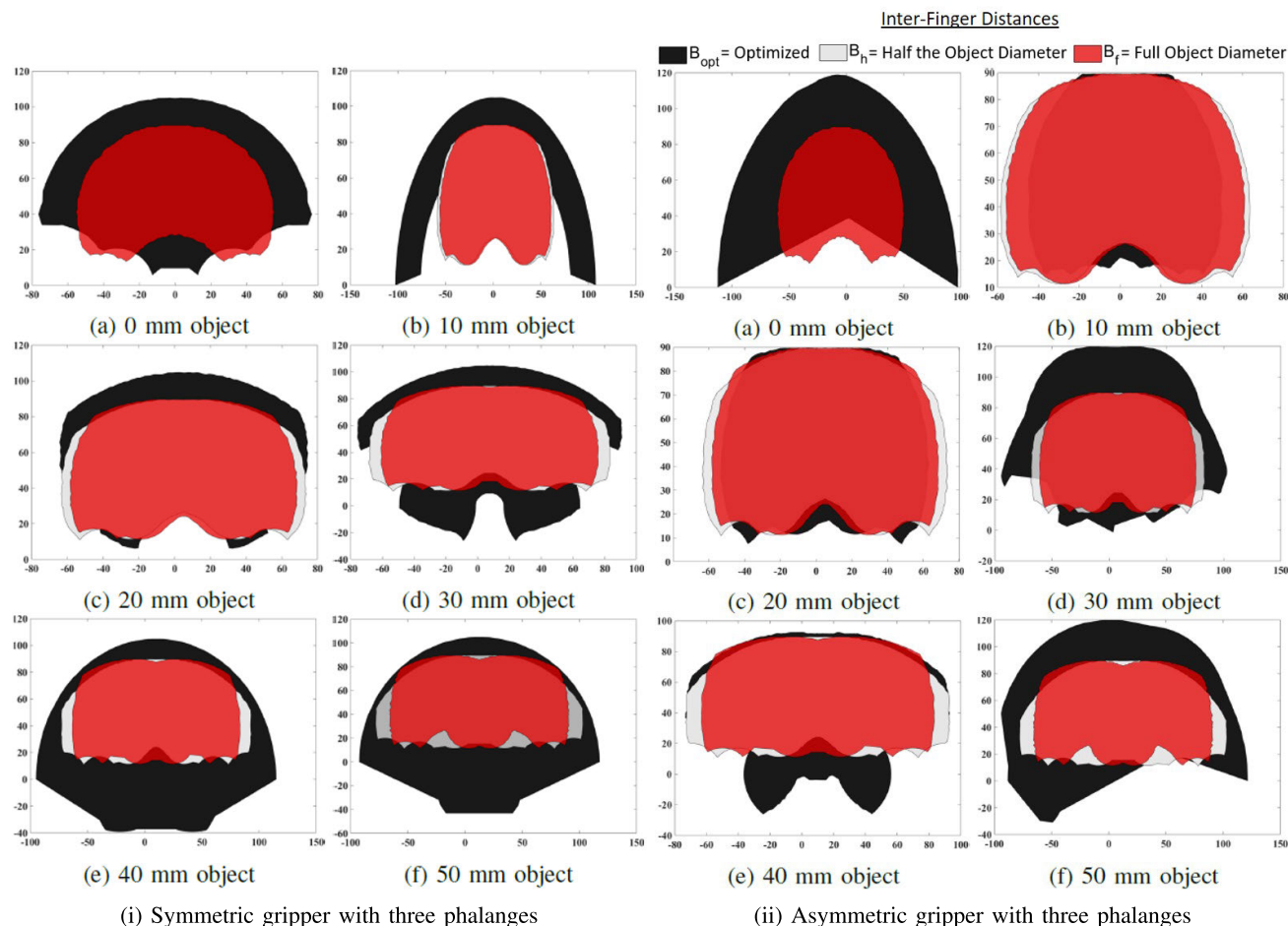
FIGURE 4. Workspace comparison results for symmetric and non-symmetric grippers with three phalanges per finger and different object diameters.
