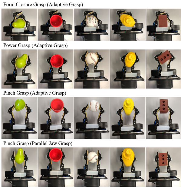
FIGURE 8. Comparison for different types of grasps that are executed with the proposed gripper.
