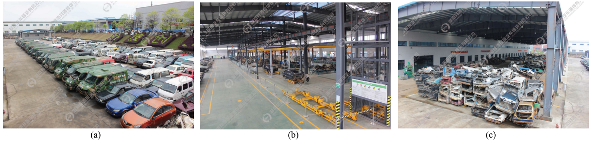
FIGURE 12. Some work scenarios of the recycling and disassembly plant; (a) recovered ELVs in warehouse; (b) semi-automatic disassembly line in disassembly workshop; (c) ELVs wreckage to be crushed in shredding workshop.
