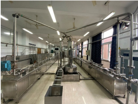
FIGURE 20. Physical drawing of gas liquid two phase flow experimental platform.
