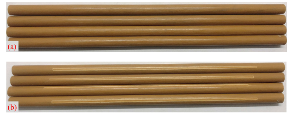
FIGURE 10. Comparison of CFRP core test samples before and after test.
