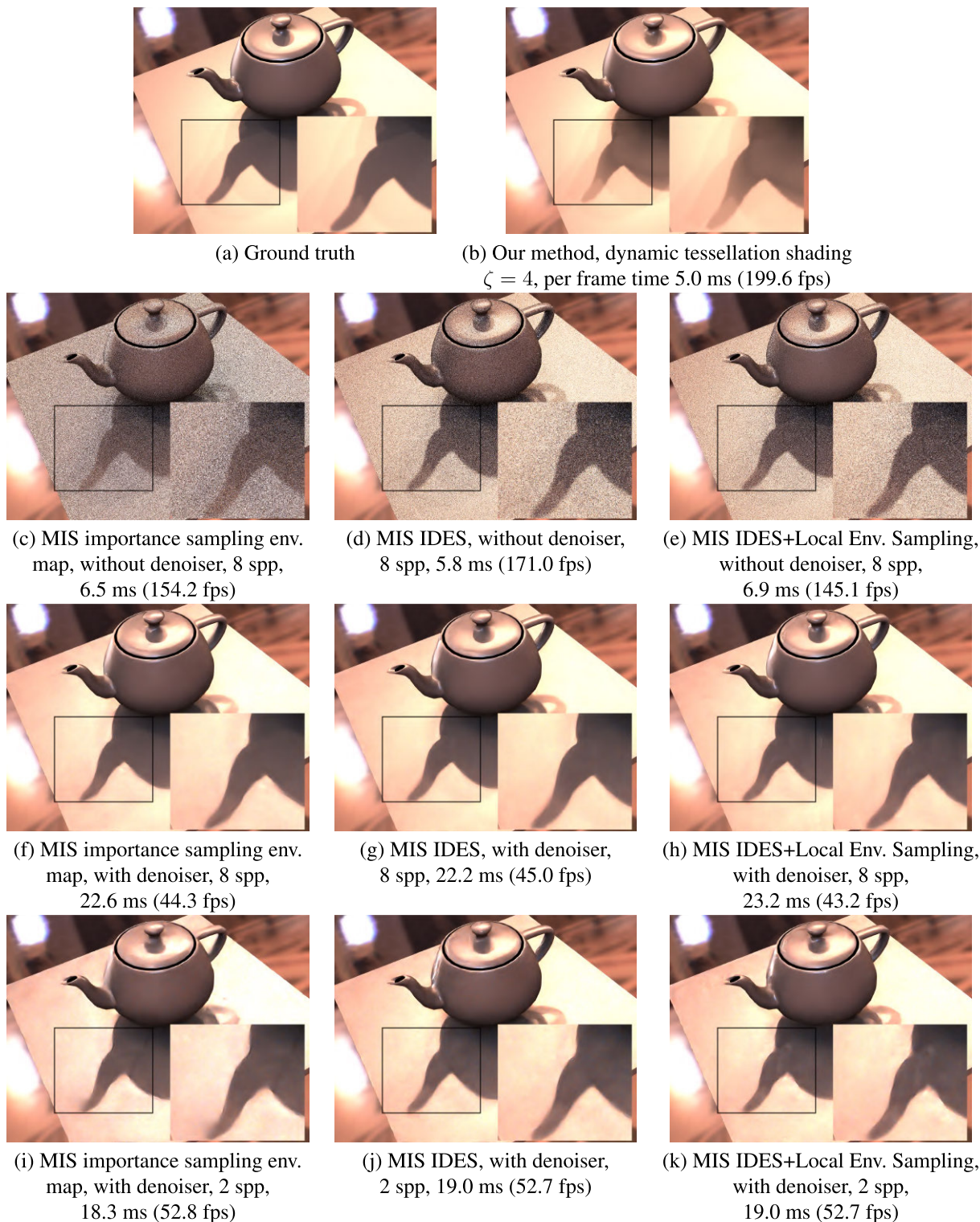
FIGURE 17. The visual evaluation for our method and the six Monte Carlo comparison targets. Given 5 ms per frame, the rendering result of our method (b) is smooth and preserves the fidelity of shadows. On the other hand, the rendering result of MIS IDES at 8 spp (d) still has a significant amount of pepper noise. Therefore, our method provides a large margin of performance improvement, i.e. 14.24 dB in terms of PSNR. With the denoiser, the rendering result of MIS IDES at 2 spp (j) has a similar PSNR as (b). However, similar PSNR only reflects similar visual quality from macroscopic point of view, which does not necessarily imply an equivalent visual quality. For instance, (b) captures local features like the subtle shadow transitions, which are lost in (j) because of not enough spp.
