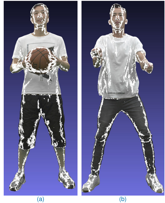
FIGURE 9. Updated 3D points in V-PCC grid-based refining segmentation. White color represents points that are associated with refined PPI. (a) Basketball player (b) Dancer player.
