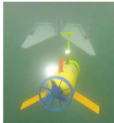
FIGURE 2. Example of landing docking [28].
