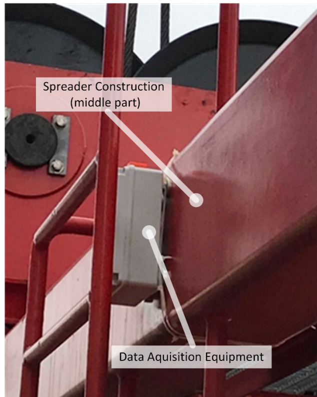
FIGURE 2. Placement of the data acquisition sensory hardware on the quay crane spreader.
