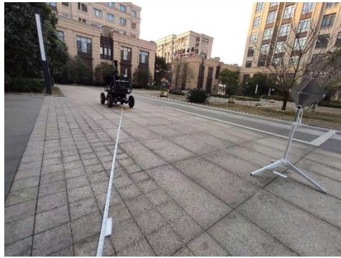
(a) Calibration using a radar angle reflector
