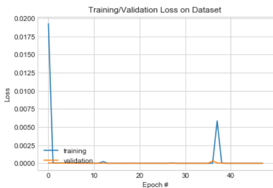
FIGURE 17. Pattern of change in loss function of training and validation on the combined dataset using Adam optimizer.
