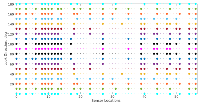
FIGURE 8. Optimal locations for a sparse array with 21 sensors on the grid of a 57-sensor full ULA for look directions 0^\circ to 180^\circ . The filled circles indicate sensor locations.
