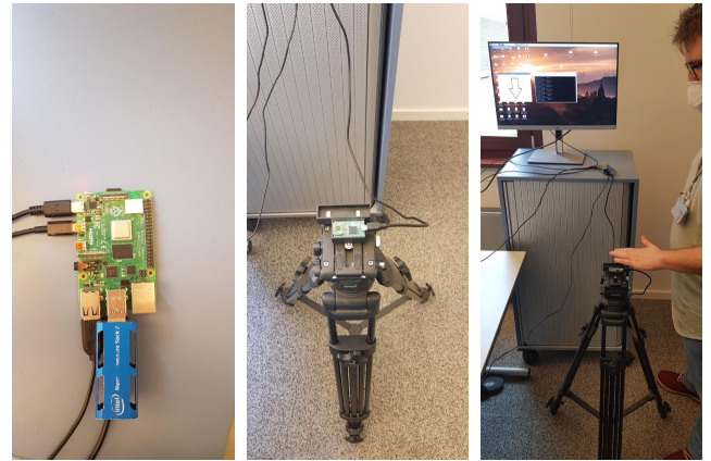
(a) Raspberry Pi4 with NCS 2 (b) Tripod with the case and Radar Sensor (c) Experimental Setup
