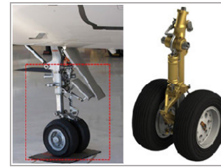
(a) Application of hydraulic parts in aircraft landing gear
