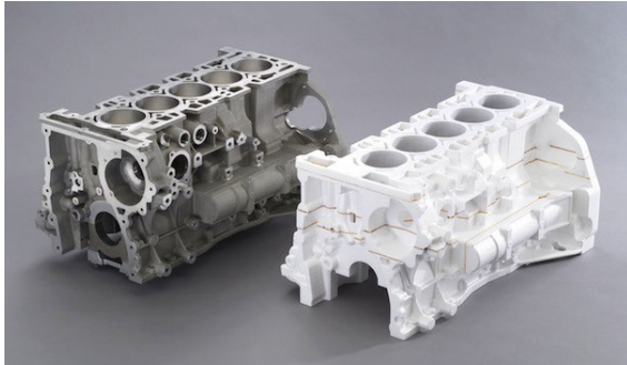
FIGURE 4. Engine foam pattern and its final casting [42].
