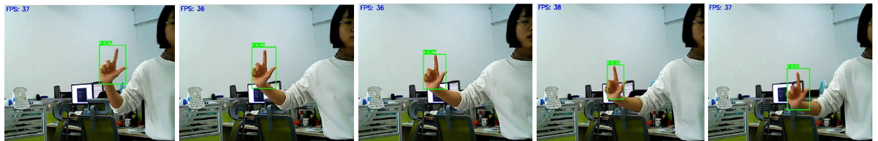
FIGURE 10. Some frames captured during real-time gesture recognition through SF-FCNet on the video.
