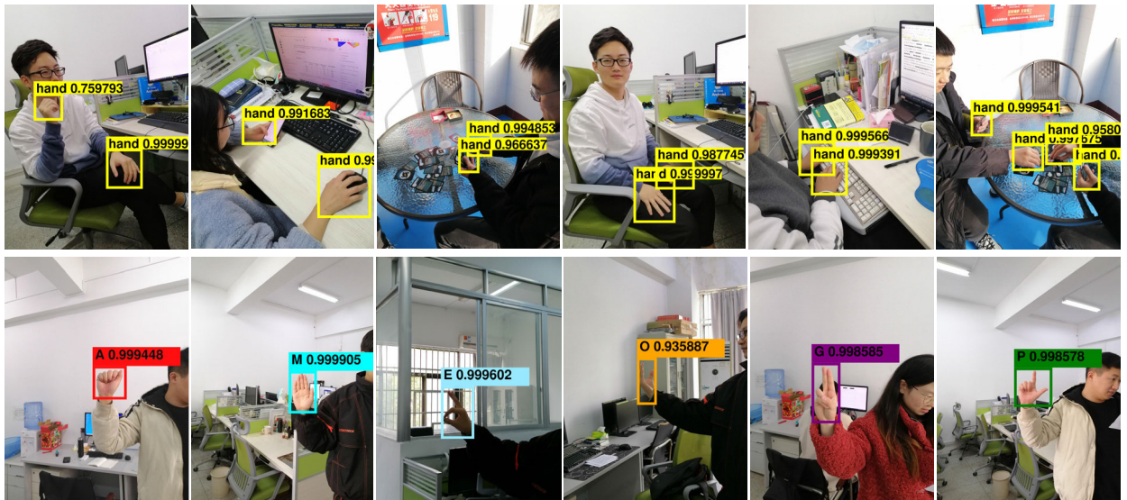
FIGURE 9. The hand detection and gesture recognition results of SF-FCNet on the homemade test set. The first row is hand detection, and the second row is gesture recognition.
