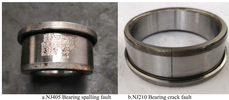
FIGURE 16. Bearing fault status.
