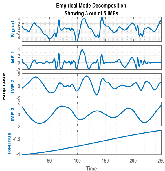
FIGURE 4. Empirical mode decomposition components from the inertial data.
