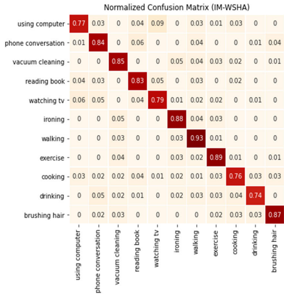
FIGURE 14. Confusion matrix of 11 different human locomotion activities on the IM-WSHA dataset using Kernel Sliding Perceptron.
