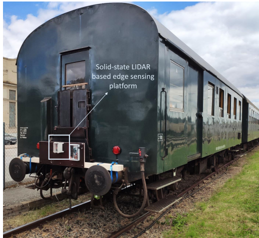
(a) Installation of the distance detection system in train A.
