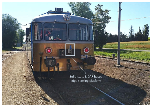
(b) Installation of the distance detection system in train B.
