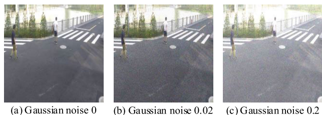
FIGURE 8. (a) Is the original frame, and frames (b) and (c) are added with different Gaussian noise.
