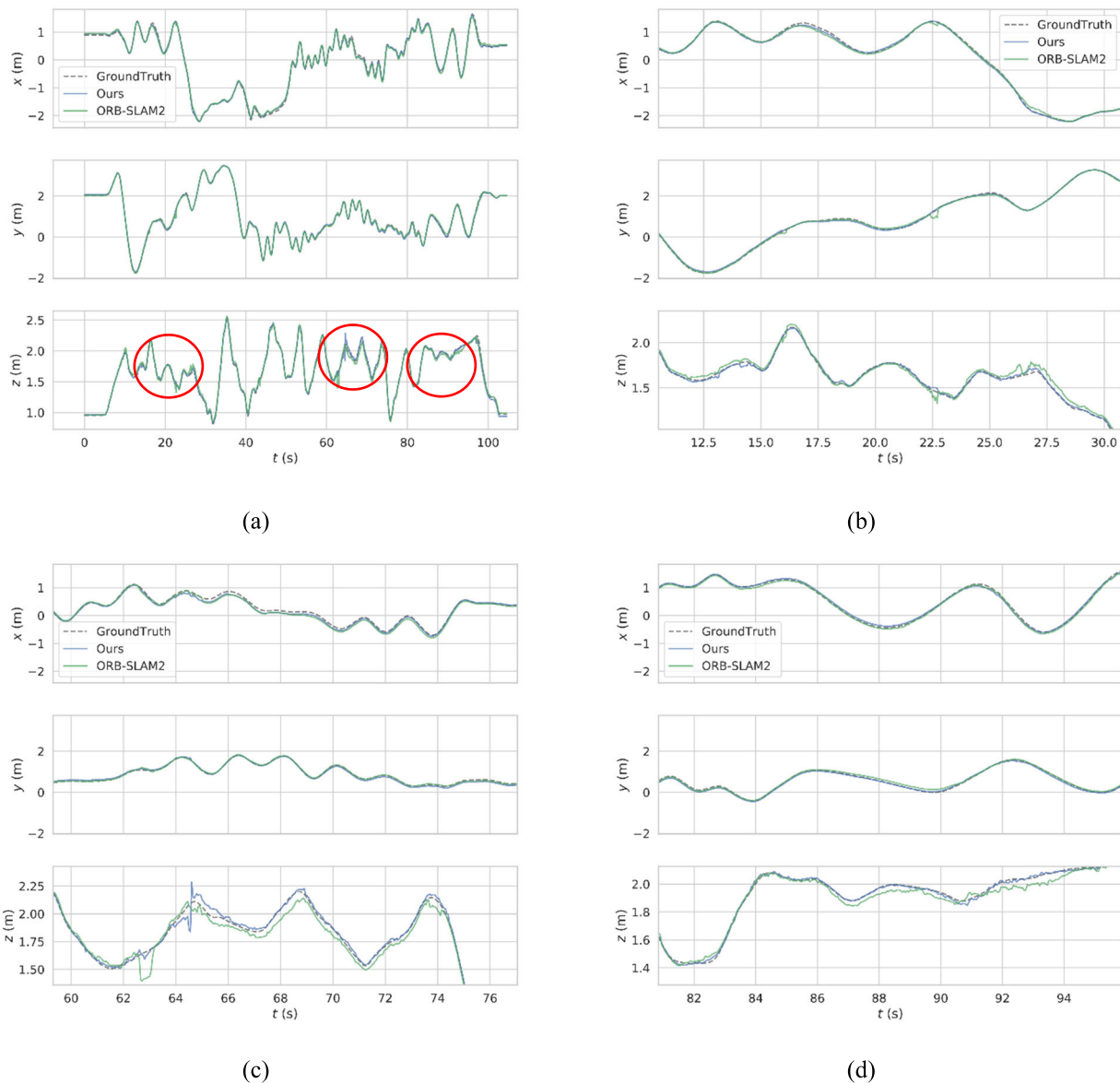
FIGURE 11. Error variation graph and enlarged graph in each axis of xyz. (a) Variation of the estimated trajectories of our algorithm and ORB-SLAM2 under the three directions of the xyz axis. We have used red circles and circled three places from left to right for the analysis. (b) Enlarged view of the first red circle. (c) Enlarged view of the second red circle. (d) Enlarged view of the third red circle.
