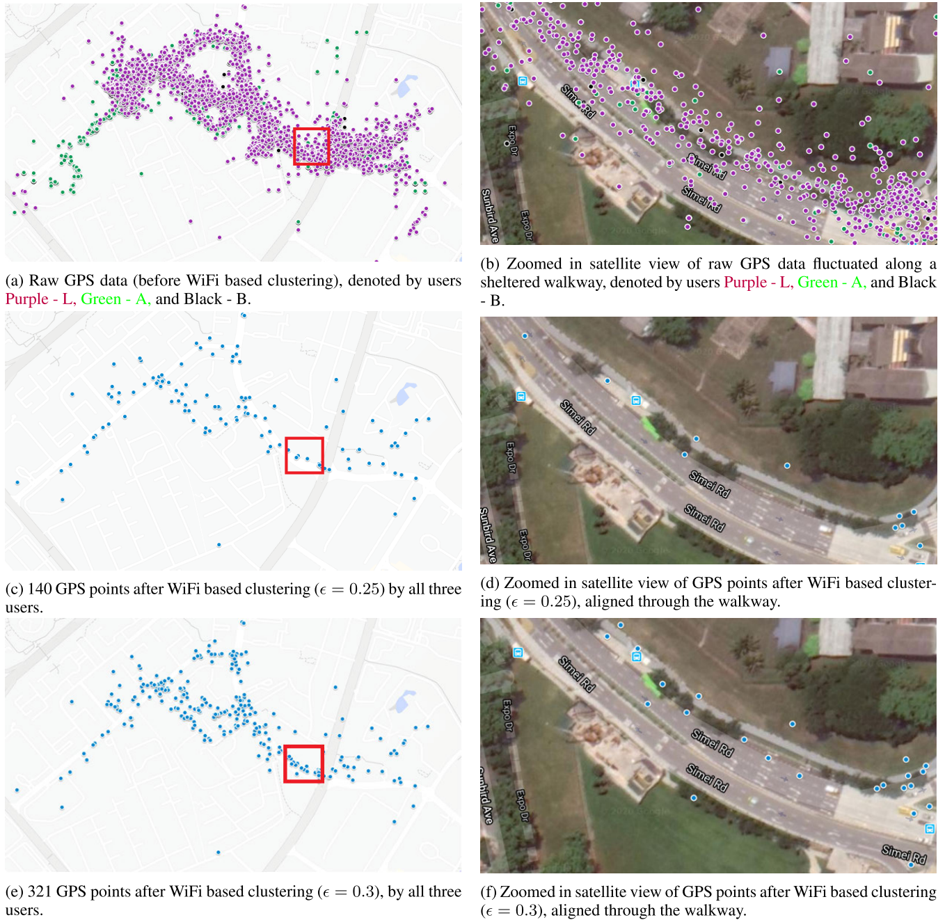
FIGURE 10. Comparison of before and after WiFi based clustering for different threshold values. 8345 points are reduced into 140 points ( \epsilon = 0.25 ) and 321 points ( \epsilon = 0.3 ).
