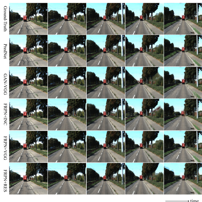
FIGURE 6. Qualitative results of multi-step video prediction on KITTI database (Inc means InceptionNet, VGG means VGGNet and Res means ResNet).
