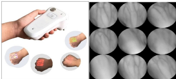
FIGURE 3. Display of dorsal hand veins in the back of the hand with infrared camera s.
