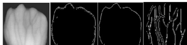
FIGURE 4. From left to right, the gray image of the hand and its veins, the image of the edge and our area of interest with Sobel edge, the extraction of the segmentation of interest or ROI by filling the cavities, the extraction of the veins of the hand, respectively.
