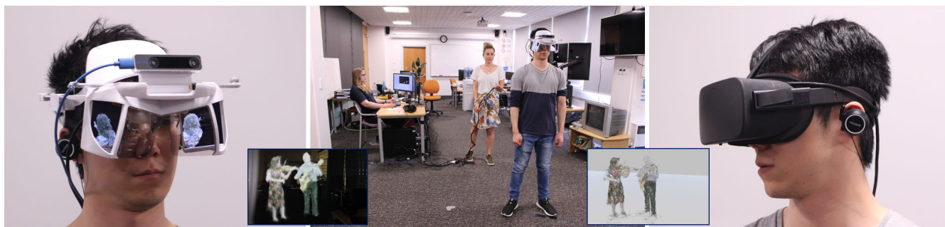
FIGURE 1. Playback of voxelvideos in laboratory environment (centre) experienced in AR (North star HMD left) or VR (Oculus rift HMD right).
