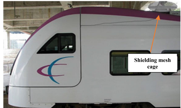
FIGURE 17. A shielding mesh cage installed on top of the array antenna which act as EMI radome.
