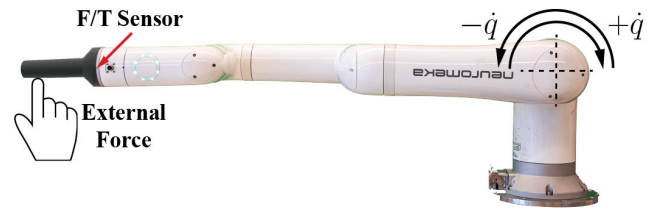
FIGURE 5. Indy-7 collaborative industrial robot: Measurement scheme to identify the load-dependent friction parameters for joint 2, and experimental conditions used to verify the teaching method.
