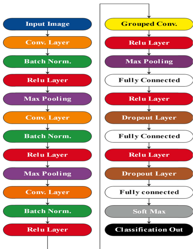
FIGURE 4. The full construction of the CNN.
