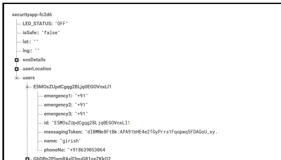
FIGURE 5. Structure of the cloud database for wearable and mobile application.
