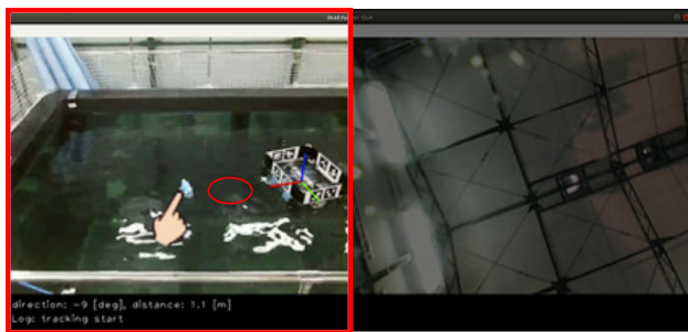
(a) Step 1: Press the target to approach it until the red circle turns green.
