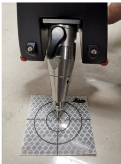
FIGURE 3. The way in which the laser tracker aimed at the reflector via the handheld T-probe.
