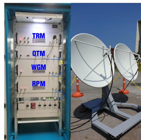
FIGURE 6. The implemented photonic radar for low-RCS target detection and image acquisition.
